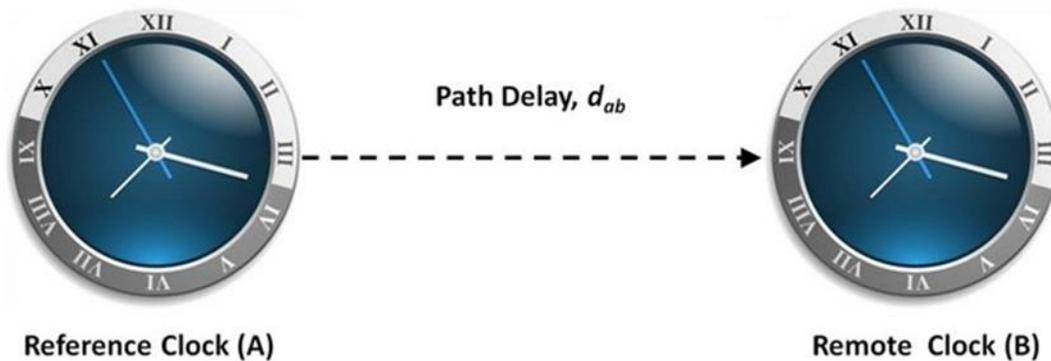
Fig. 1. A simple “one-way” time transfer system.
