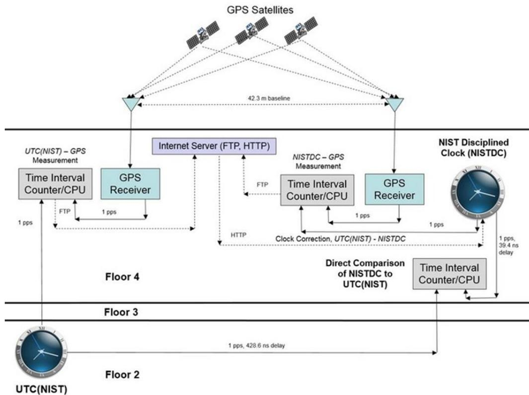
Fig. 4. Measurement configuration for direct comparison of a NISTDC to UTC(NIST).
